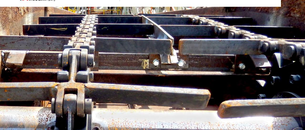
A Brazilian manufacturer of OSB and MDF wood-based products used enmasse conveyors to move raw materials from off-load to distribution and manufacturing. Poor design and small conveyor size—complicated by incorrect flight selection—meant the conveyors could not handle the required loads or the characteristics of the material.
