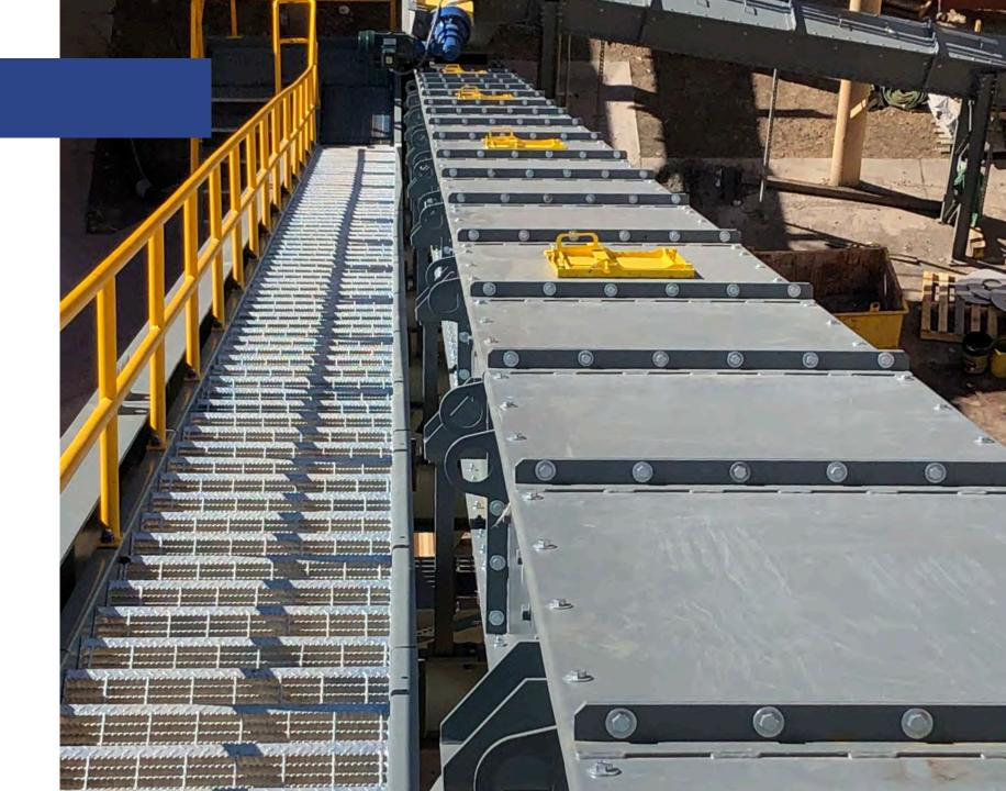
CDM's exclusive CrMn forged steel alloy chains have a core hardness of 300-400 BHN and are machined and carburized for a case of 550-650.
