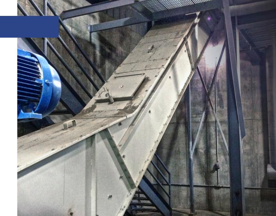
The two conveyors allowed the facility to have built-in redundancy and continuously supply fuel to the boilers.
