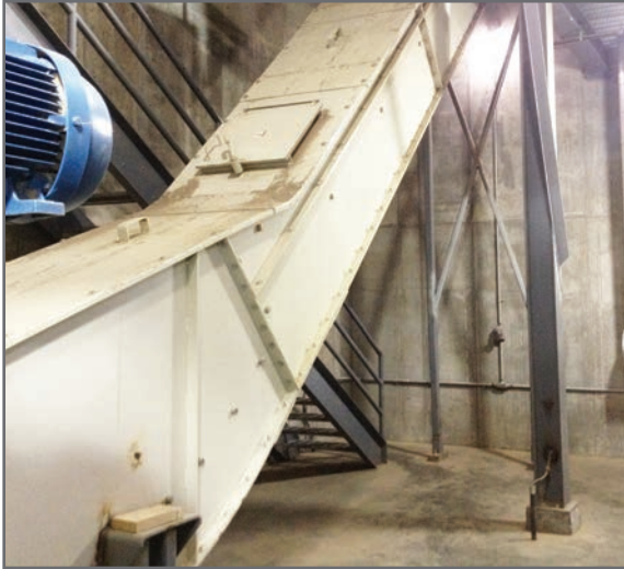
L Path Conveyor design minimized chain pull and maximized conveyor life.
