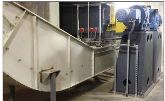
The En-Masse Drag Chain Conveyor receives biomass material directly from the in-feed hopper. The sealed drag chain carries material up to the storage silo.
