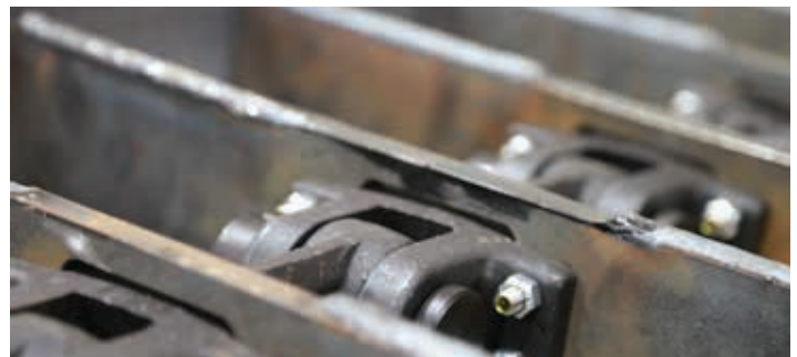
FIGURE 6 CDM SYSTEMS CONVEYOR CHAIN
